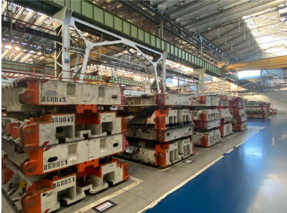
Figure 14: Series of dies outside production line (Stellantis data)
