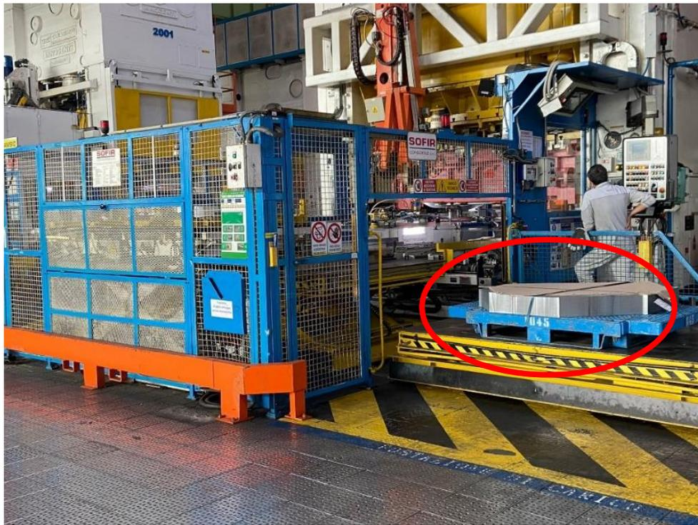
Figure 13: Feeding the Pressing line with metal sheets (Stellantis data)
